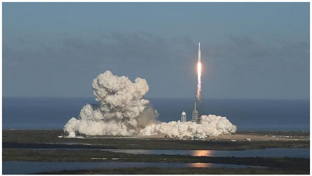
Propelled by 27 rocket engines, the Falcon Heavy packs more than 5 million pounds of thrust at launch, roughly three times the force of the Falcon 9 booster rocket that until now has been the workhorse of the SpaceX fleet. The new heavy-lift rocket is essentially constructed from three Falcon 9s harnessed together side by side.
